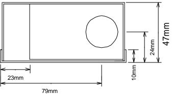
Fixing Holes 2 off M3 Clearance holes marked 'A'
